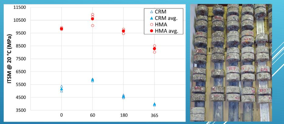
For both mixtures a gradual increase in stiffness from day 0 to 60 was followed by a reduction trend until day 365 The initial rise of the stiffness moduli is probably due to the road pavement settlement given by traffic. After 60 days a gradual decrease in stiffness is recorded: loss of mechanical properties of the layer due to the combined effect of traffic and climate.
