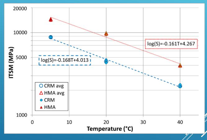
Thermal sensitivity was assessed testing at 5, 20 and 40 ° C Stiffness values are higher for Hi-HMA at all temperatures The 2 mixtures show similar variation of stiffness with temp.
