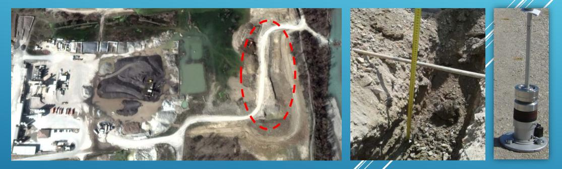
A 60 cm thick layer, characterised by a measured Light Weight Deflectometer Modulus (ELWD) of 70 MPa, was considered as foundation for the trial road section. The foundation was very well compacted by local heavy dumpers traffic.
