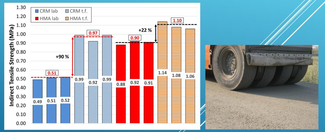
The histogram shows higher ITS for cores than laboratory specimens (+90 %). The ITS values of CRM are very high considering this type of AC and are similar to those usually obtained from common bituminous mixtures.
