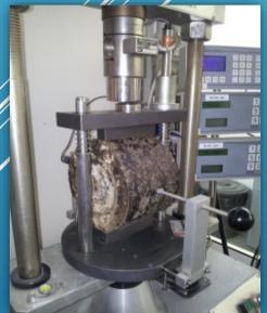
The ITS for CRM is higher than ITS (limit (0.35 MPa) imposed by some Italian technical specifications for CMA for base layer. Notice: these limits are related to mixtures made with less than 30 % of RAP.
