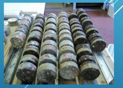
If compared to the volumetric analysis made during the laboratory phase, it can be observed that the air voids content is lower for the core samples.
