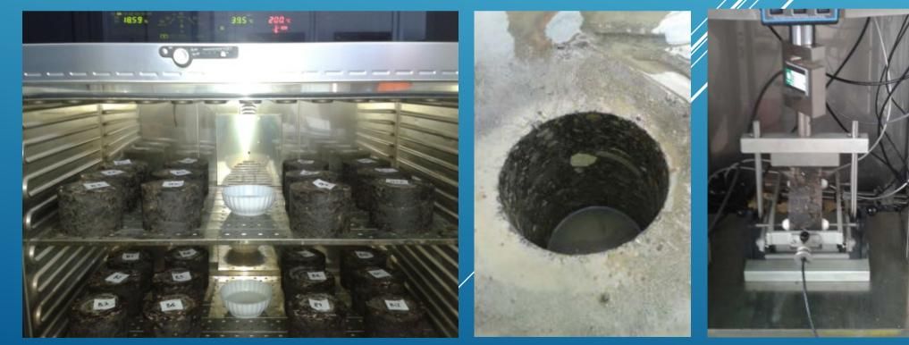
3 compacted samples for each loose mixture were prepared by gyratory compaction at day 0.
