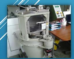
Air voids (EN 12697-8) are in line with those recommended for base layers. Compactability is generally one of the weakest points for CRM, if compared to the traditional hot mixing technique.
