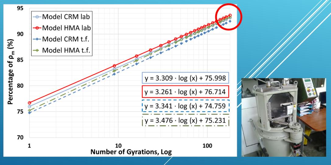
No substantial differences between the compaction curves of the CRM and HMA produced in plant.
